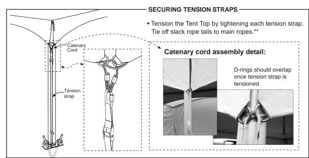
**IMPORTANT:** Each installation site must be evaluated by installer to determine proper securing method. Site conditions may require guying and/or anchorage different from what was provided with the structure.
