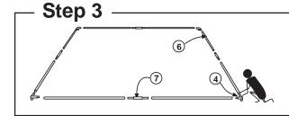
• Assemble Corner 90° (4), Eve Tubes (6), Mid Joints (7) by slipping one part to another to form the eve frame.
